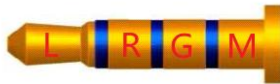
Figure 15 Definition of four-segment headphones
