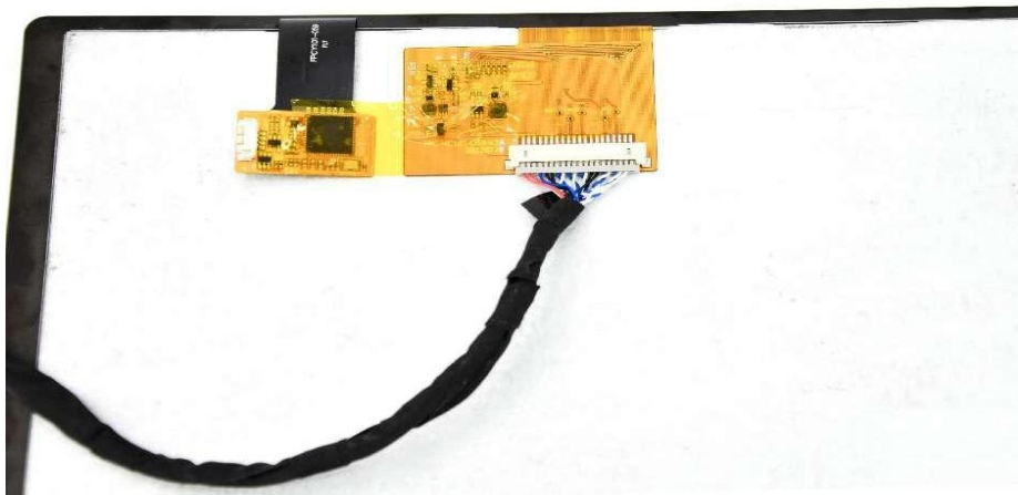
Figure 31 Connect LVDS screen cable to LVDS screen
